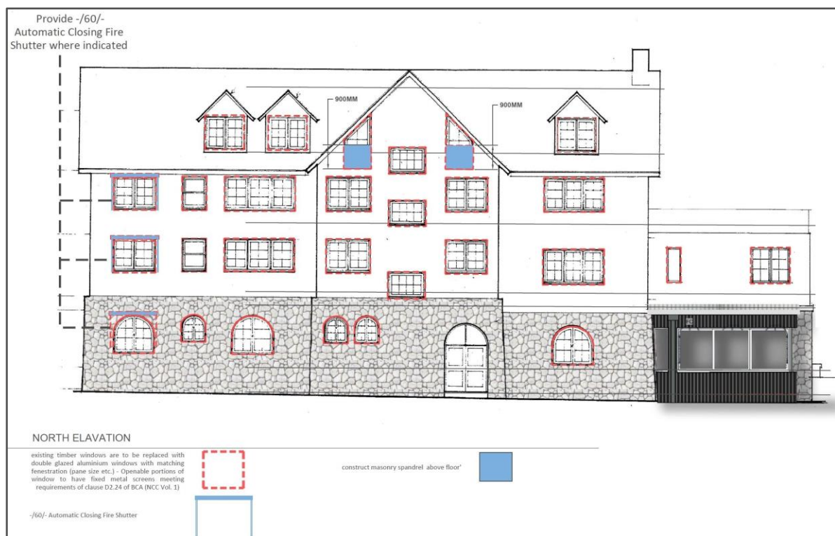
Figure 3 | Existing North Elevation, with windows to be replaced (red dotted) and spandrel works in blue (Source: Applicant's documentation)
